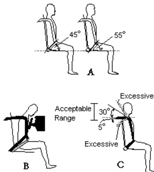
The end attachments of the shoulder harness must also be installed at appropriate angles. The ideal position is anywhere between  $5^\circ$  below and  $30^\circ$  above the driver's shoulder, as seen in part C of the Figure.
