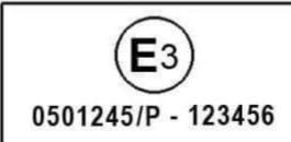
An ECE approved helmet can be recognized by the label on the chin strap, which consists of a large E in a circle with a number, the number corresponding to a country. UK is E11, Italy is E3, and so on.
