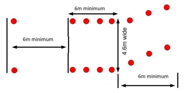
The end of the course must be made into a finish box consisting of at least 14 cones arranged in the shown shape. Note: The minimum distance from the stop line to beginning of stop box is 45 meters (49 ft) 6m (20ft) while the stop box must be a minimum of 6m (20ft) by 4.6m with pylons narrowing the box and indicating direction to leave the course for an additional 6m (20ft). Total stop box length is 15m 12m (49ft).
