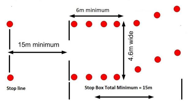
The end of the course must be made into a finish box consisting of at least 14 cones arranged in the shown shape. Note: The minimum distance from the stop line to beginning of stop box is 15 meters (49 ft) while the stop box must be a minimum of 6m (20ft) by 4.6m with pylons narrowing the box and indicating direction to leave the course. Total stop box length is 15m.
