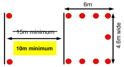
The end of the course must be made into a finish box consisting of at least nine (9) cones arranged in the following shape. Note: The minimum distance from the stop line to beginning of stop box is 15 meters 10m (33ft) while the stop box must be a minimum of 6m (20ft) by 4.6 m. The outer perimeter of the stop box is a line connecting the outside edges of the end and side pylons
