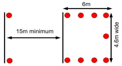
The end of the course must be made into a finish box consisting of at least nine (9) cones arranged in the following shape. Note: The minimum distance from the stop line to beginning of stop box is fifteen meters while the stop box must be a minimum of 6m by 4.6 m. The outer perimeter of the stop box is a line connecting the outside edges of the end and side pylons.
